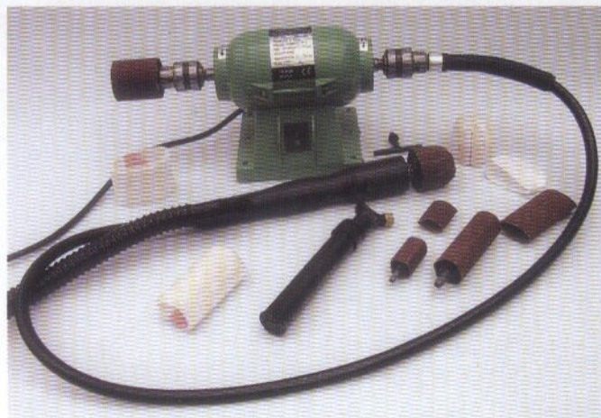
The power unit with the flexible drive and integrated dust collection system, with the dome sander fitted. In the other chuck is a cylinder sanding unit. The pump, polishing and abrasive sleeves are in front of the motor
